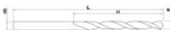
19 HSS-E5 metal drill bit (5% cobalt) - SLR graduated - Split point - Ø 1 to 10 mm by 1/2
